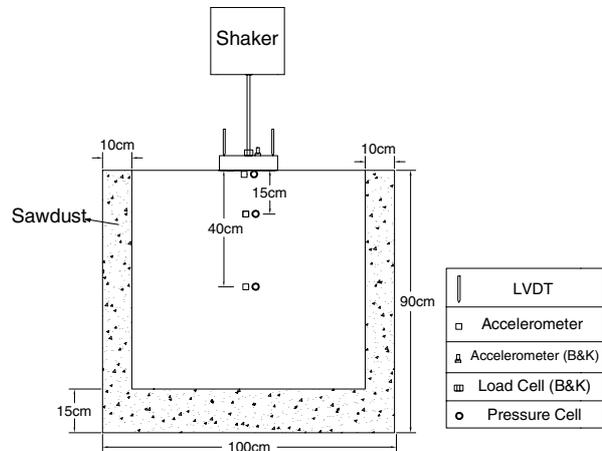
Figure 1. Schematic experimental set up of physical models.
