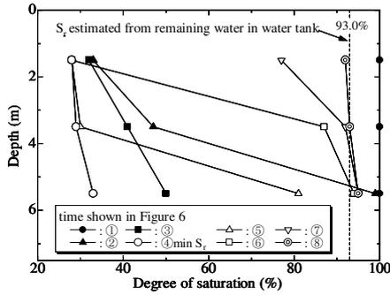
Figure 7. Depth profile of degree of saturation in desaturation process: U15.
