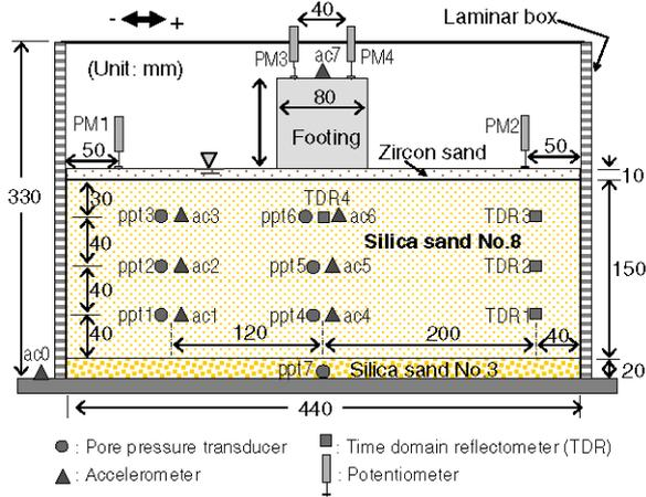
Figure 5 (a). Test setup and location of sensors in the model.
