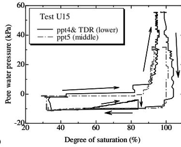
Figure 8. Variation of pore water pressure with  $S_r$ .
