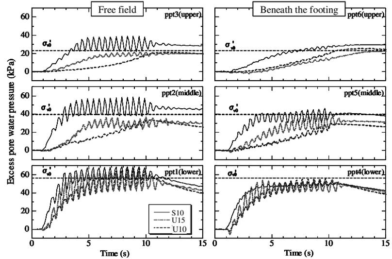
Figure 11. Variation of excess pore pressure in the model ground during shaking.
