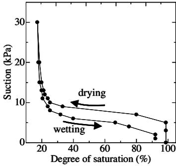
Figure 2. Capillary pressure and degree of saturation curve : Silica sand No.8.
