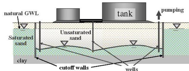
Figure 1. Desaturation of liquefiable soils by groundwater lowering.
