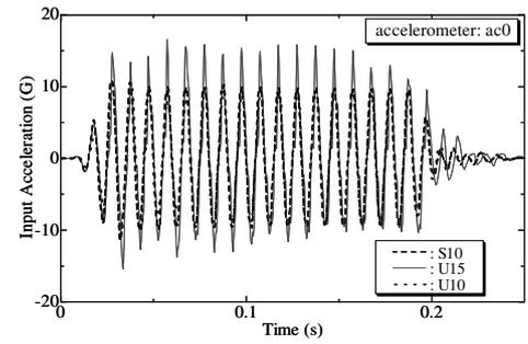
Figure 9. Input base acceleration measured by acc0.
