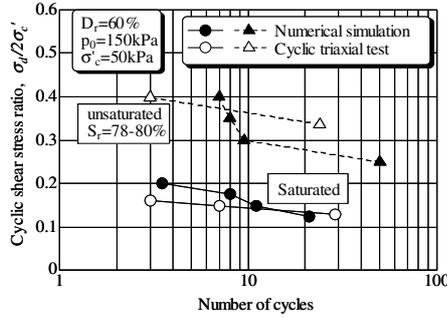
Figure 3. Relationship between cyclic stress ratio and number of cycles: Silica sand No.8.
