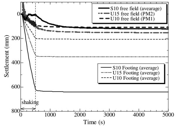
Figure 14. Settlements of the footing and free field during and after shaking.
