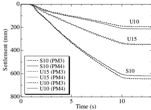
Figure 12. Settlements of the footing during shaking.
