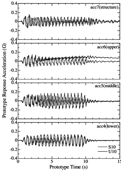
Figure 10. Observed acceleration beneath the footing.
