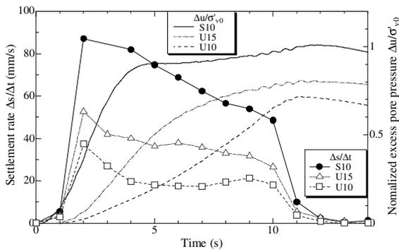
Figure 13. Variation of settlement rate of footing and normalized excess pore water pressure (PPT5) during shaking.
