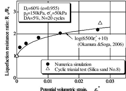
Figure 4. Relationship between potential volumetric strain and liquefaction resistance ratio.
