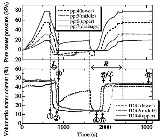
Figure 6. Variation of pore pressure and volumetric water content in desaturation process: U15.
