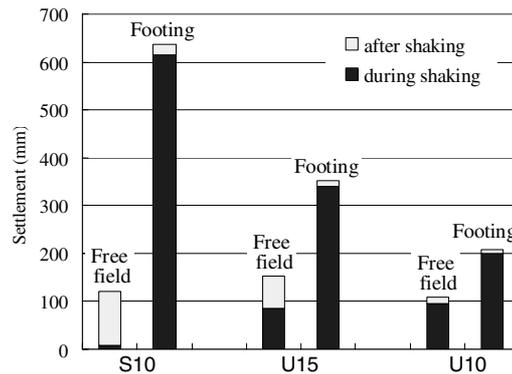
Figure 15. Settlements of the footing and free field.
