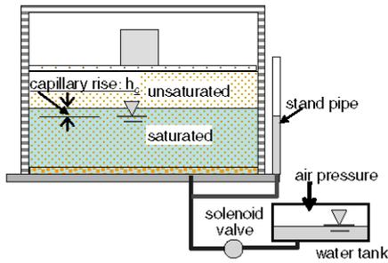
Figure 5 (b) Control of ground water level in the model.
