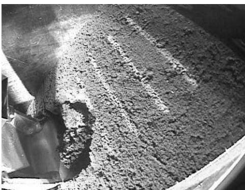
Figure 12 Slope failure event in the model slope Case-C2
