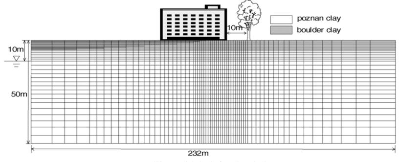
Figure 3 Mesh for simulation
