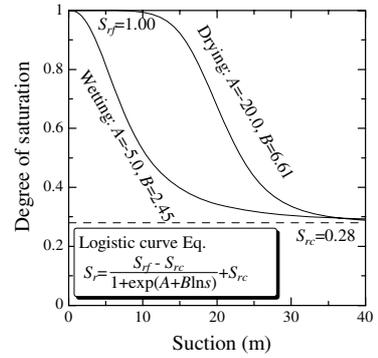
Figure 7 Soil-water retention characteristic
