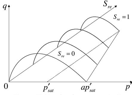
Figure 1 Yield surface for unsaturated soil
