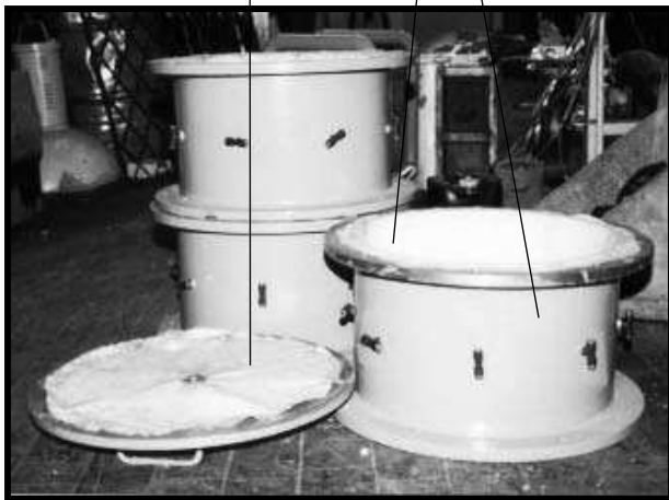
Figure 1. Triaxial test tank.
