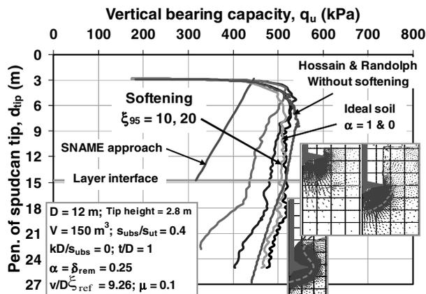
Figure 4. Comparison among LDFE results, Hossain & Randolph approach and SNAME approach (double layer clay).
