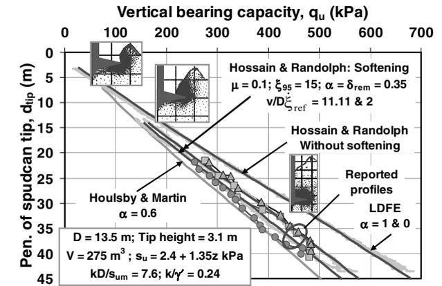
Figure 3. Comparison among LDFE results, Hossain & Randolph approach, SNAME approach and reported field data (single layer clay). [Rate effect:  $\mu$  is relative strength change per decade of strain rate change; softening:  $\xi_{95}$  is cumulative plastic shear strain for 95% remoulding,  $\delta_{rem}$  is inverse of soil sensitivity.]
