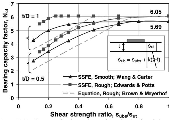
Figure 2. Bearing capacity factor for surface circular foundation on stiff-over-soft clay ( $kD/s_{subs} = 0$ ).
