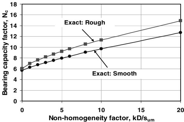
Figure 1. Bearing capacity factors for surface circular foundation for different  $kD/s_{um}$ .
