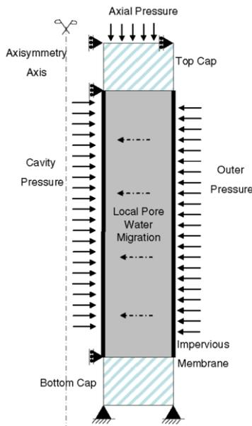
Figure 4. A schematic diagram showing the numerical model used in TWC simulations
