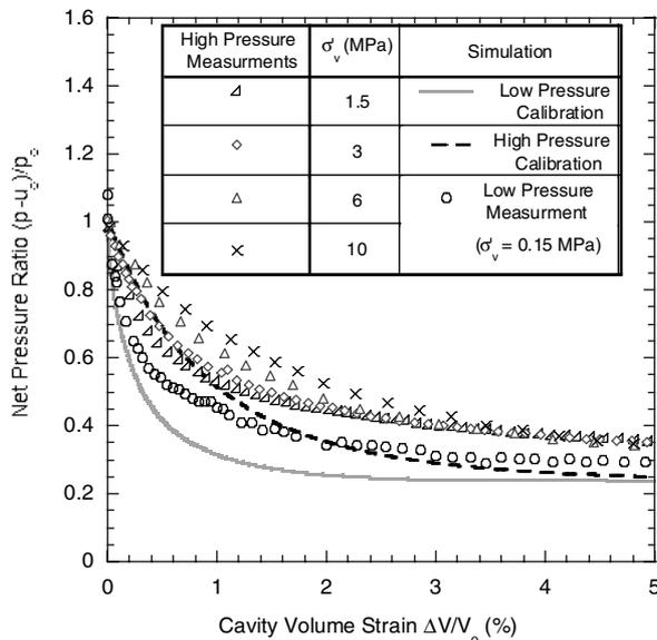
Figure 5. FE simulations compared to TWC lab results.
