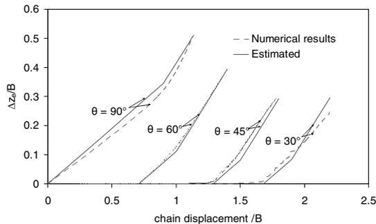
Figure 7 Loss of anchor embedment correlating to chain displacement
