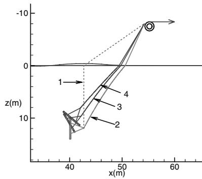
Figure 5 Anchor and chain position during pullout in FE analysis
