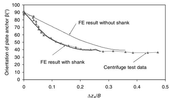
Figure 4 Comparison between FE results and transparent soil test data
