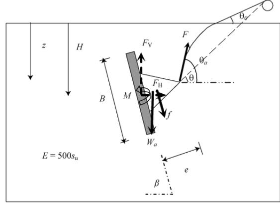
Figure 2 Setup of anchor in numerical analysis
