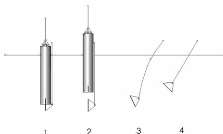
Figure 1 Installation and anchor keying processes for the Suction Embedded Plate Anchor (SEPLA)
