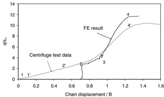
Figure 6 Pullout responses in FE analysis and transparent soil
