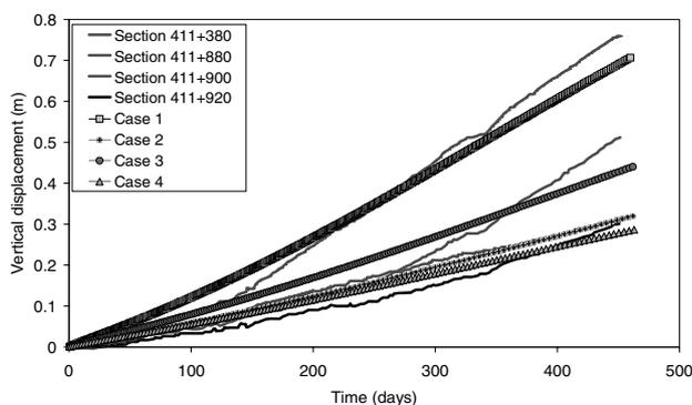
Figure 9. Calculated (Case 1 to 4) and measured vertical strains (Sections) on the flat-slab surface of Lilla tunnel.
