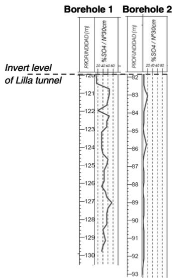
Figure 6. Sulphate proportion in the rock from a borehole located near a tunnel section with maximum (left) and minimum swelling phenomena (right).
