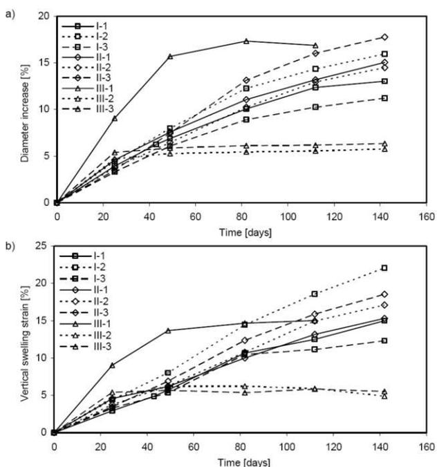
Figure 5. Swelling records for the tested specimens during free swelling tests. a) Diameter increase. b) Height increase (Oldecop 2006).
