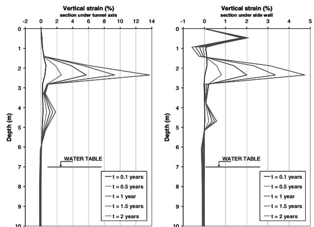
Figure 8. Vertical strains in two vertical sections. A) Under tunnel axis; B) Under the side wall.
