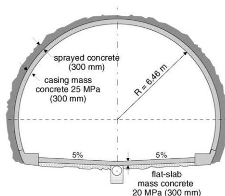
Figure 1. Original cross-section in Lilla tunnel.
