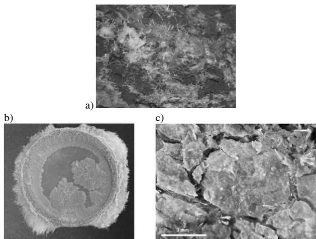
Figure 3. a) Gypsum needles on an open slickensided surface located in the active zone. b) Gypsum crystal growth on the surface of a powdered compacted sample, bottom face (Berdugo 2007). c) Evidences of degradation due to crystal growth on a sample at the end of a drying test (Oldecop 2006).
