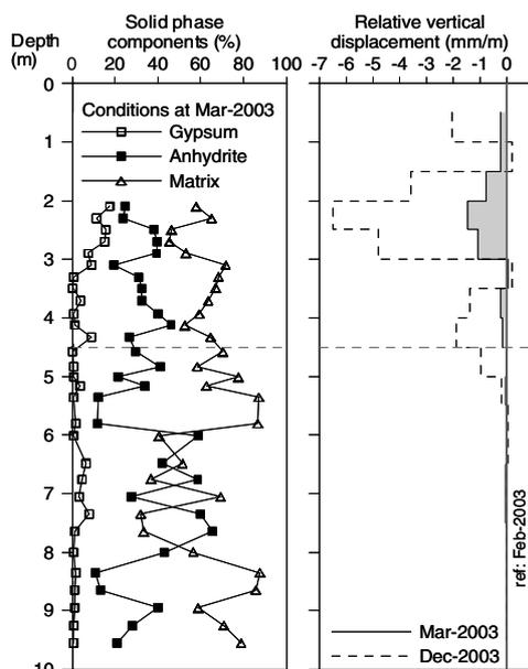
Figure 4. Characterization and vertical expansive profile of station 411+600 (invert-arch).
