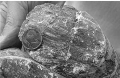
Figure 7. Slickensided surface from Borehole 1 in Lilla tunnel.
