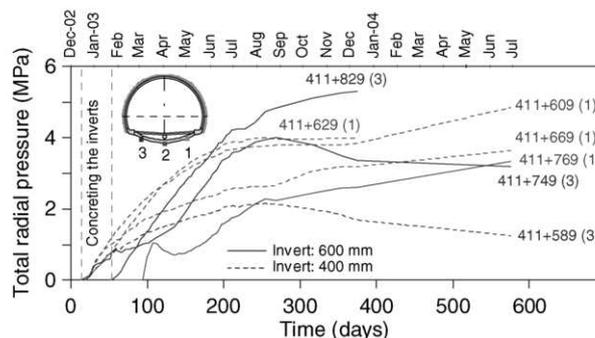
Figure 2. Evolution of total radial stress in test sections with invert-arch.
