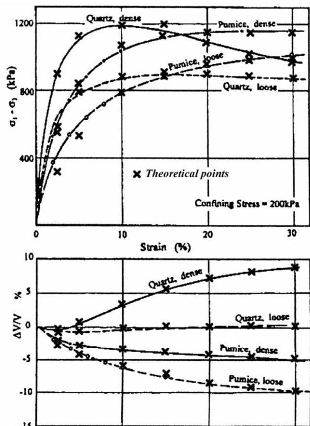
Figure 1. Typical Triaxial Behaviour of Pumice & Quartz Sands
