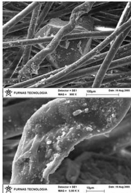
Figure 6: Large entrapped tailings particles in the geotextile pores.
