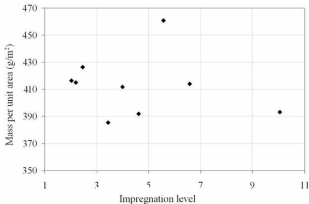
Figure 7: Level of impregnation versus mass per unit area for the exhumed geotextile sample.
