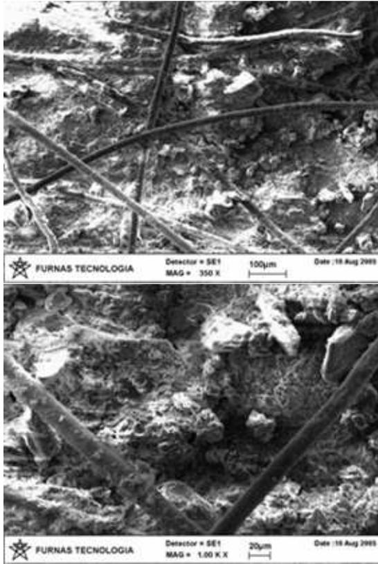
Figure 4 - Particles clusters close to the geotextile surface.
