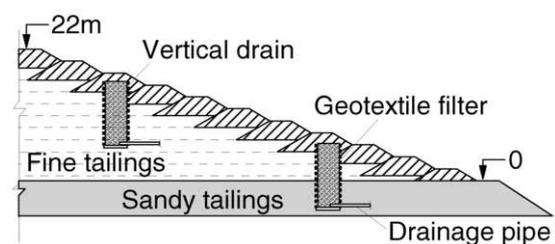
Figure 1. Vertical drains – Drying bays of the Germano Dam.
