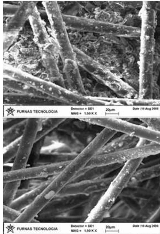
Figure 5 – Particle clusters inside the geotextile.
