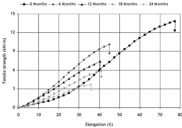
Figure 2. Mean curves tensile strength-elongation obtained for GTX B before and after natural weathering.
