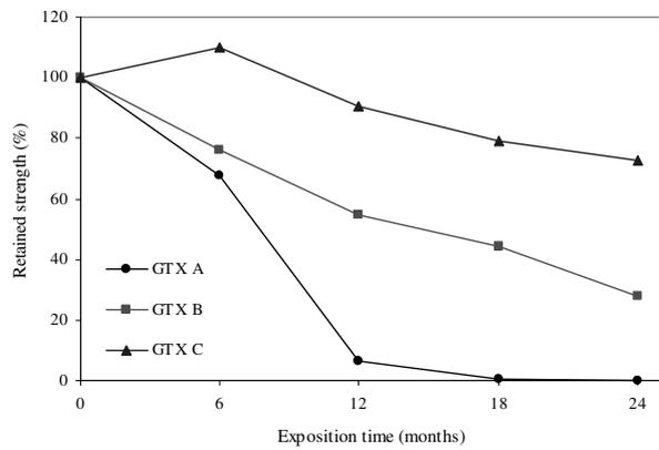
Figure 3. Evolution of the retained strength of the GTXs A, B and C during the natural weathering tests.
