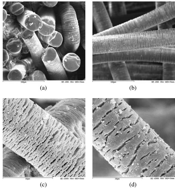
Figure 4. SEM photographs of the GTXs after exposition to natural weathering: (a) and (b) GTX A after 12 months (x500); (c) GTX B after 24 months (x2000); (d) GTX C after 24 months (x2000).
