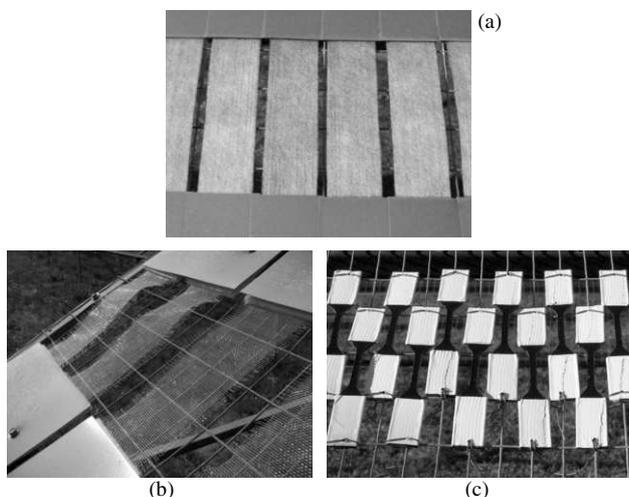
Figure 1. Geosynthetic samples exposed to natural weathering: (a) geotextiles; (b) geonets; (c) geomembranes.
