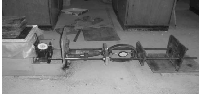
Figure 1. Pull-out test apparatus
