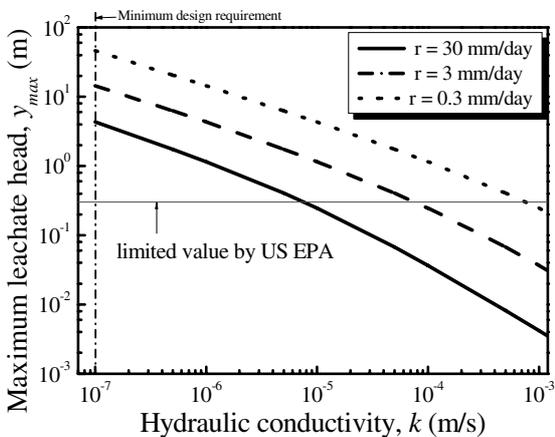
Figure 2. Calculated maximum leachate head versus hydraulic conductivity of granular drainage materials
