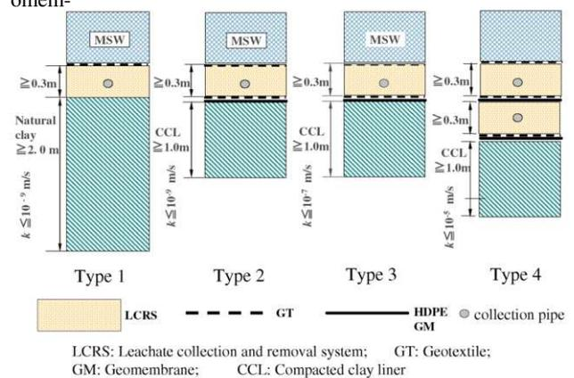
Figure 1. Illustration of Chinese standard landfill liner system
