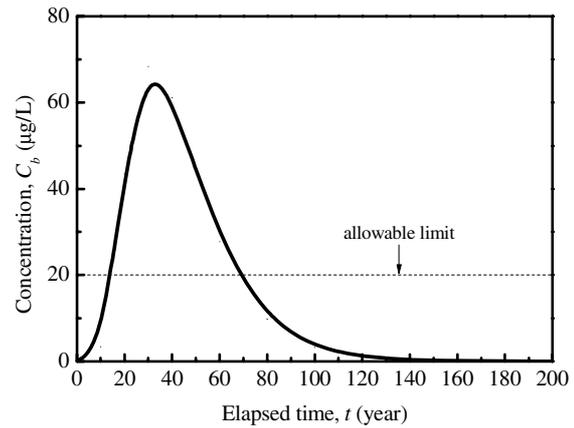
Figure 6. Change of calculated concentration at aquifer with time for CN 1 liner
