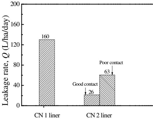
Figure 5. Calculated leakage rate through CN 1 &amp; CN 2 liners
