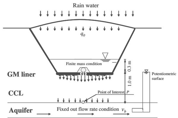
Figure 4. Assumed landfill in which CN 2 liner is used
