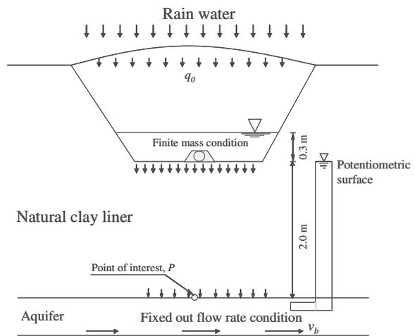
Figure 3. Assumed landfill in which CN 1 liner is used
