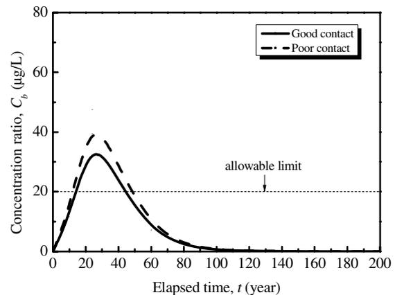
Figure 7. Change of calculated concentration at aquifer with time for CN 2 liner
