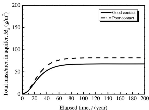
Figure 9. Change of total mass per unit are discharged into aquifer with time for CN 2 liner
