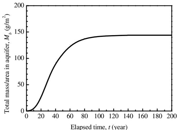
Figure 8. Change of total mass per unit are discharged into aquifer with time for CN 1 liner
