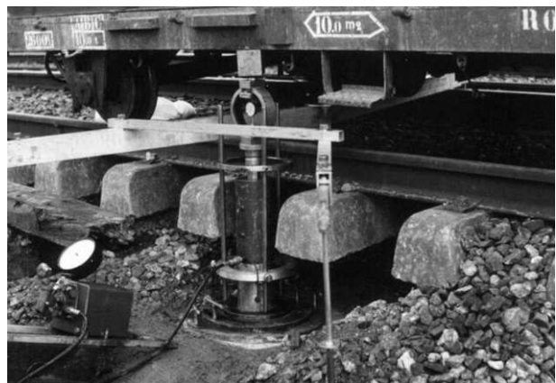
Figure 1. Plate Load Test during survey of railway subgrade
