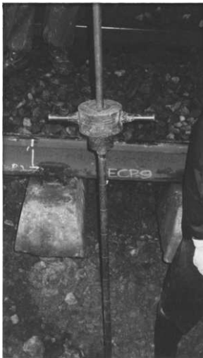
Figure 2. DCP during field survey of the old railway platform
