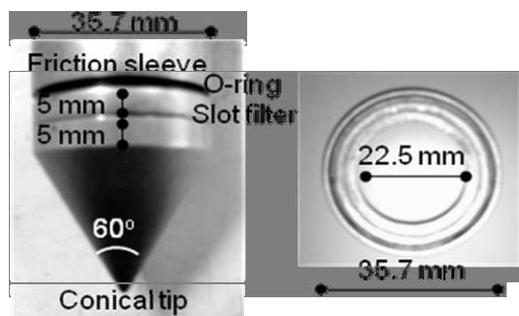
Figure 1. Detail of the piezocone tip and slot filter.
