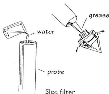
Figure 2. Piezocone saturation procedure using slot filter (SGI 1995).
