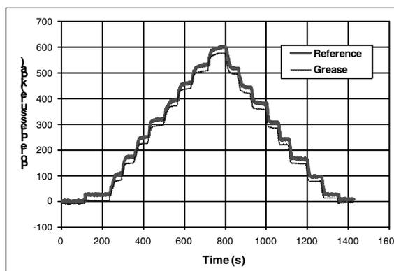
Figure 5. Pore pressure versus time curves using slot filter with grease.
