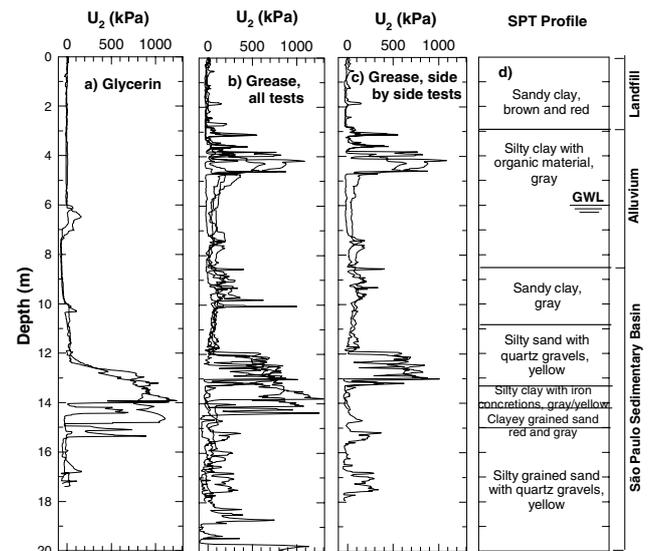
Figure 9. Pore pressure records from piezocone tests using grease and glycerin for São Paulo-SP site, including side-by-side testing data.
