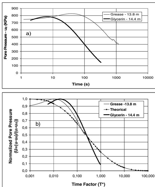
Figure 10. Pore pressure dissipation curves for São Paulo-SP site using glycerin and grease. Side by side tests.
