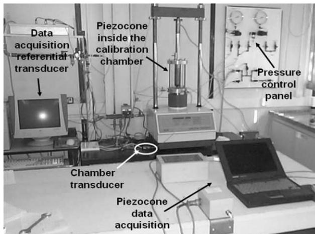
Figure 3. System for piezocone testing in laboratory.
