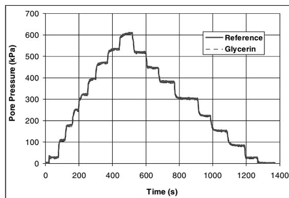
Figure 4. Pore pressure versus time curves using porous element with glycerin.
