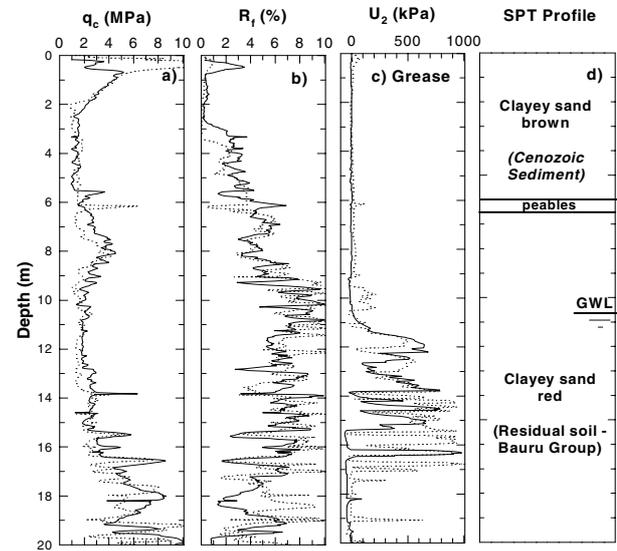
Figure 8. Pore pressure records from piezocone tests using grease for São Carlos-SP site and soil profile based on SPT.
