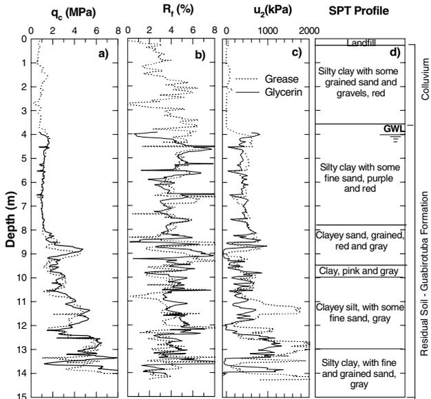
Figure 6. Side by side pore pressure records from piezocone tests using grease and glycerin for Curitiba-PR site, and soil profile based on SPT.
