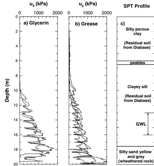
Figure 7. Pore pressure records from piezocone tests using grease and glycerin for Campinas-SP site.
