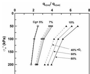
Figure 4. Effect of gypsum content, relative density, and vertical effective stress on cone tip resistance of cemented sand.
