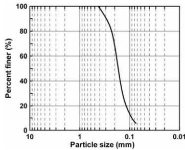
Figure 1. Particle size distribution of K-7 sand.
