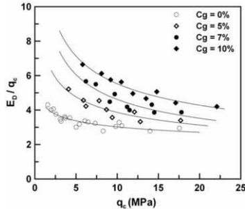
Figure 7. Effect of cementation on  $E_D/q_c$  of sand.
