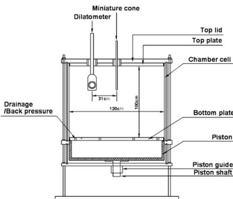
Figure 2. Calibration chamber system for CPT and DMT.
