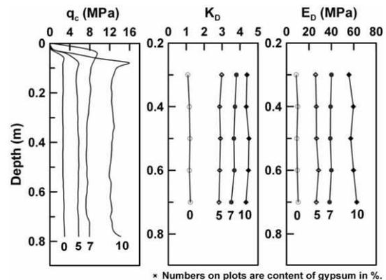
Figure 3. Typical profiles of q<sub>c</sub>, K<sub>D</sub> and E<sub>D</sub> in chamber (Dr≈40%, σ<sub>v</sub>'=100kPa).
