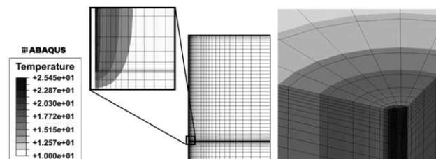
Figure 4. FE-models of a borehole heat exchanger for test interpretation; left: axisymmetric, right: tree-dimensional.
