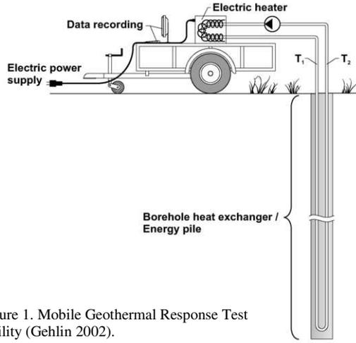
Figure 1. Mobile Geothermal Response Test facility (Gehlin 2002).
