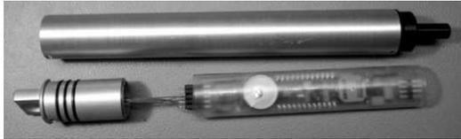
Figure 5. Wireless measuring probe (length 235mm,  $\varnothing$  23mm) called "micro fish" (Rohner et al. 2004).
