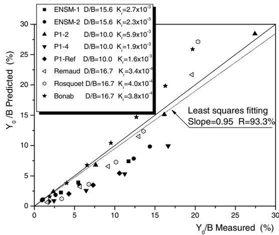
Figure 5. Comparison of ground deflection of prototype piles
