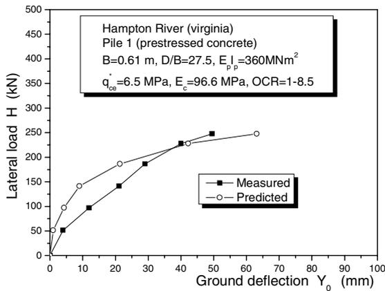
Figure 2. Comparison of load-deflection curves of full-scale tests
