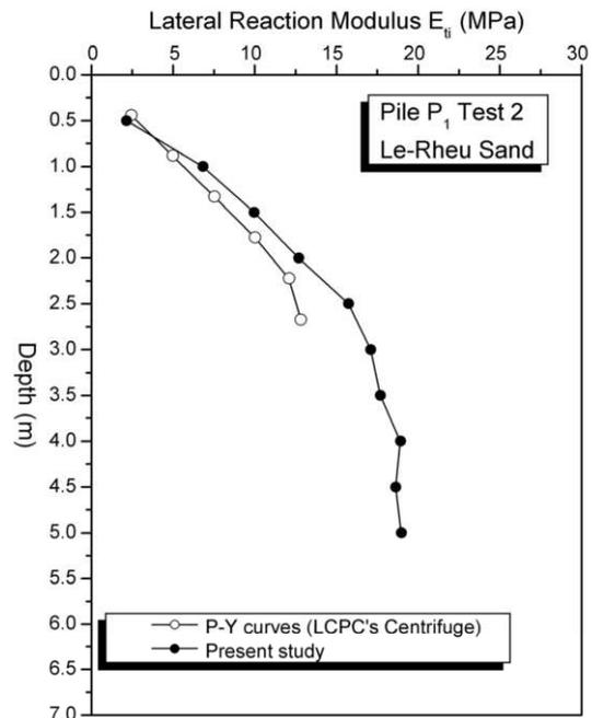
Figure 4. Comparison of the lateral reaction moduli
