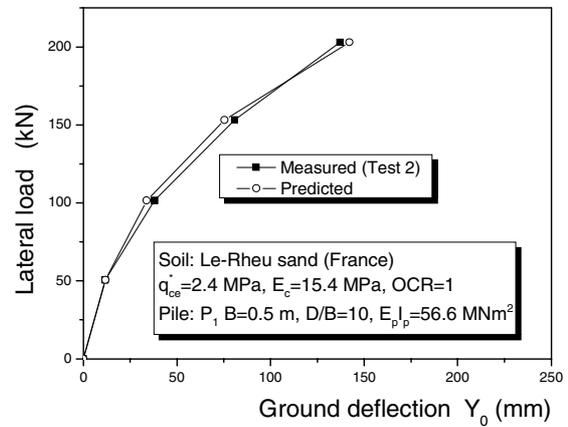
Figure 3. Comparison of load-deflection curves of centrifuge tests
