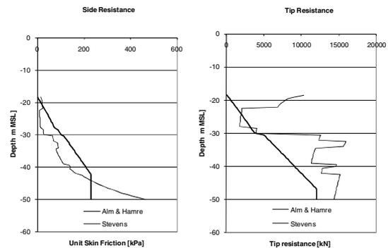
Figure 5. Soil resistance to driving
