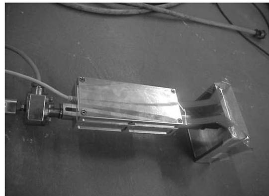
Figure 3. Model-raft with four unloaded walls, loadcell, Tekscan device.
