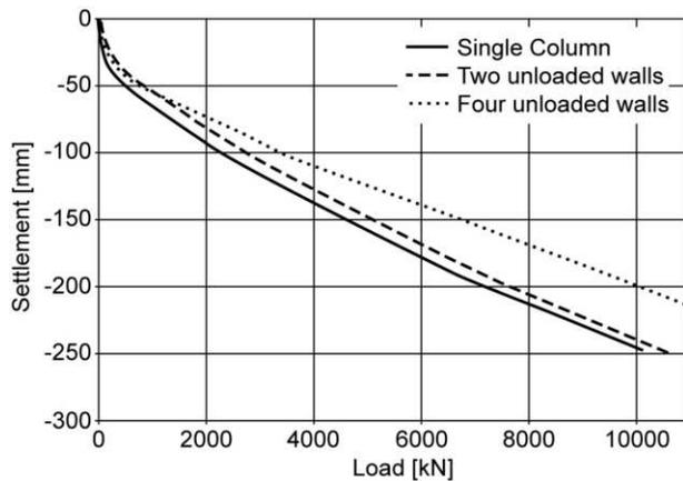
Figure 10. Load-Settlement-Behaviour for the three tests (prototype scale).
