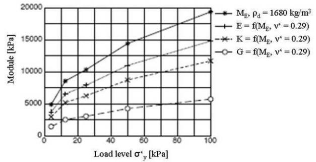
Figure 1. Soil stiffness  $M_E$  on different load levels (Nater, 2006)
