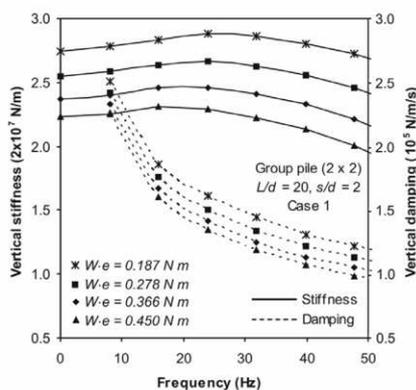
Figure 7. Vertical stiffness and damping of pile group ( $L/d = 20$ ,  $s/d = 2$ , Case 1) for different exciting moment
