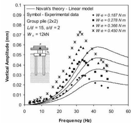
Figure 4. Comparison of experimental and theoretical (Linear model) response curves ( $L/d = 15$ ,  $s/d = 2$ ,  $W_s = 12$  kN, Case 1)
