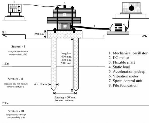
Figure 2. Schematic diagram of test setup for vertical vibration
