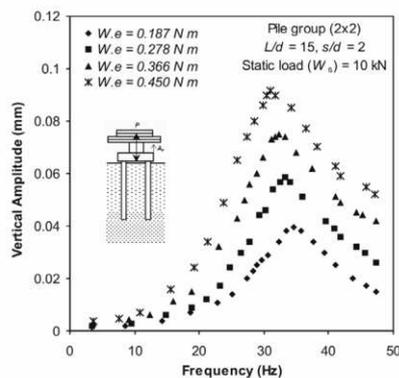
Figure 3. Experimental frequency-amplitude response curves for vertical vibration ( $L/d = 15$ ,  $s/d = 2$ ,  $W_s = 10$  kN, Case 2)
