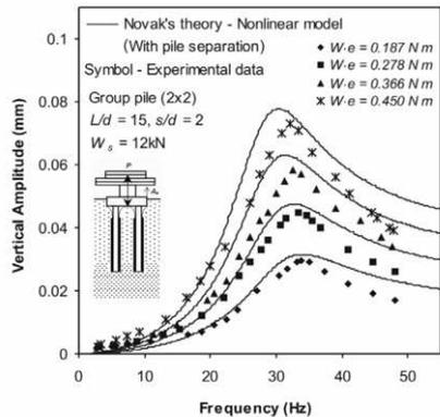
Figure 6. Comparison of experimental and theoretical (Nonlinear model) response curves ( $L/d = 15$ ,  $s/d = 2$ ,  $W_s = 12$  kN, Case 1)
