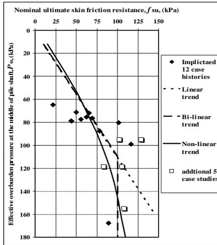
Fig. 2: Side resistance versus effective overburden pressure.
