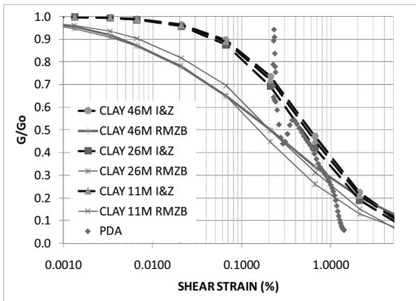
Figure 5. Dynamic stiffness degradation curves estimated for the site from the equations by Ishibashi and Zhang (I&Z), from the study for revision of the seismic microzonation of Bogota (RZMSB) and data points obtained from the PDA analysis.
