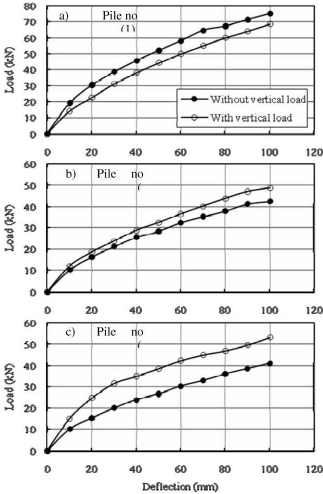
Figure 7. Group pile response: Measured and computed load versus pile head deflection curve, pile spacing/ diameter = 3.92
