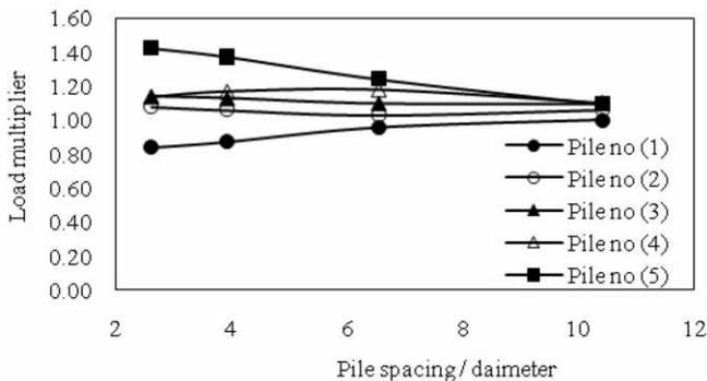
Figure 8. Load multiplier versus pile spacing to diameter ratio.
