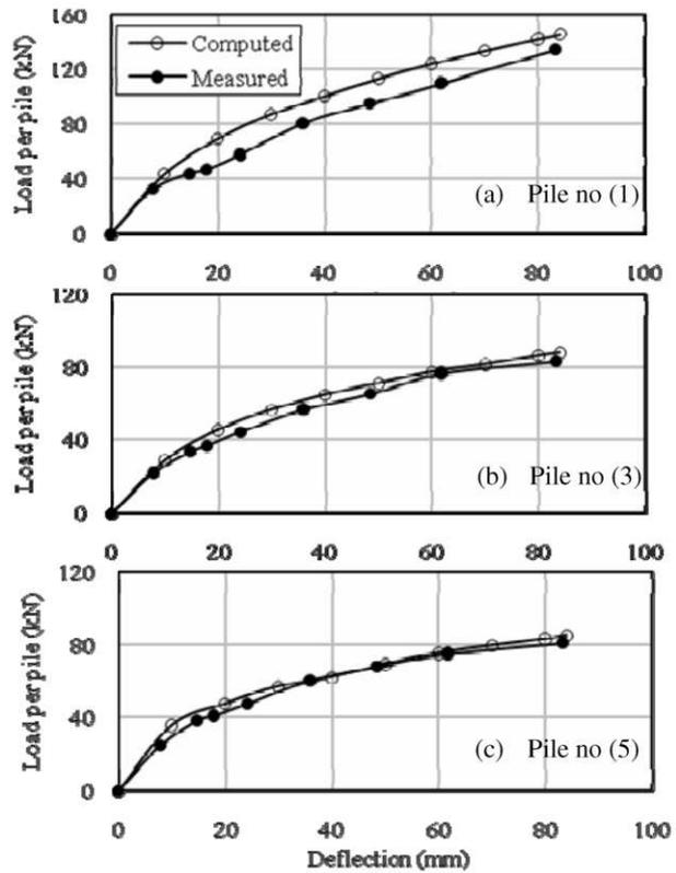
Figure 5. Group pile response: Measured and computed load versus pile head deflection of no 1, no 3, and no 5 pile
