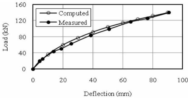
Figure 4. Single pile response: Measured and computed load versus pile head deflection curve
