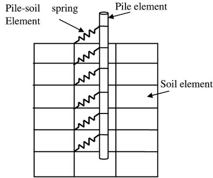
Figure 3. Concept of pile-soil spring element.
