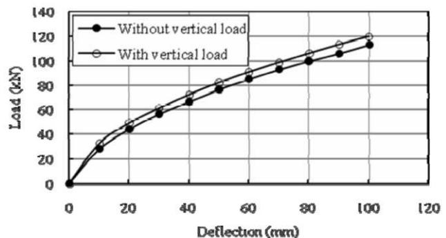
Figure 6. Single pile response: Measured and computed load versus pile head deflection curve
