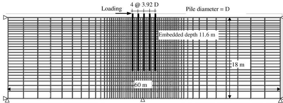
Figure 1. General layout and meshing of the FE model.
