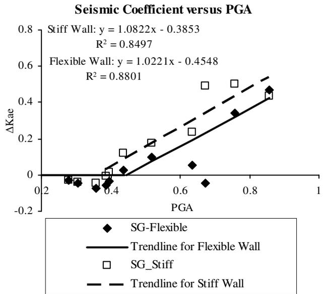
Figure 4. Seismic coefficients computed at maximum dynamic wall moments based on strain gauge (SG) data.
