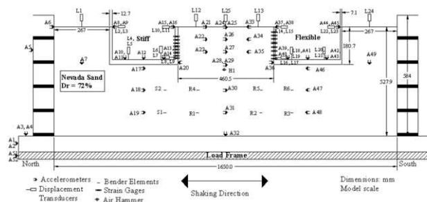
Figure 1. Section through the model showing the position of the model structures and the layout of instrumentation. Dimensions in model scale (mm).
