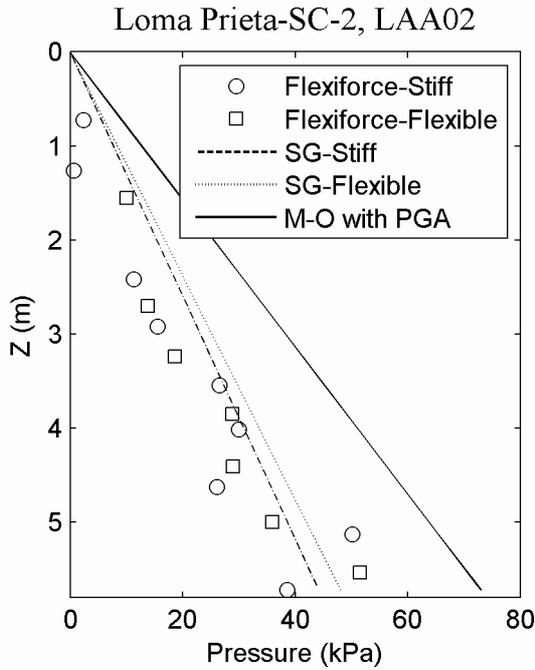
Figure 2. Maximum total earth pressure profiles measured with strain gauges (SG), tactile sensors, and estimated using the M-O method for Loma Prieta-SC-2 event (Sitar and Al Atik, 2009)
