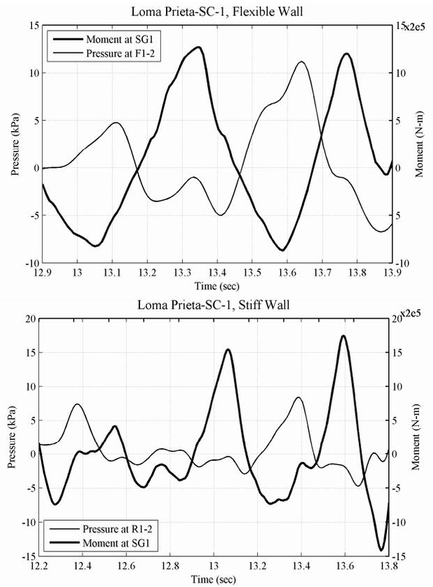
Figure 3. Comparison of dynamic wall moments and dynamic earth pressures on the south stiff and north flexible walls (Sitar and Al Atik 2009)
