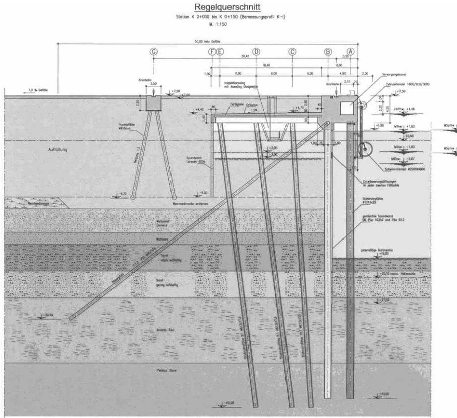
Figure 5. JadeWeserPort, tender design, cross section of the quay wall
