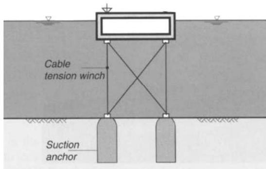
Figure 4. Floating concrete structure, anchored by suction anchors (Handbook Quay Walls)
