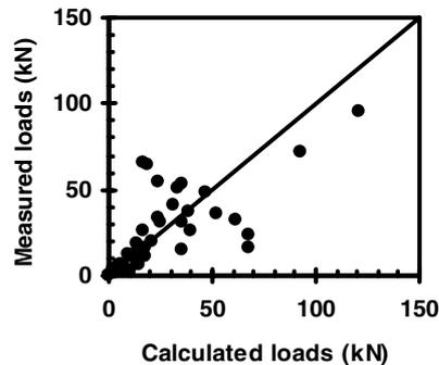
Figure 3. Comparing measured and calculated loads for steel grids.
