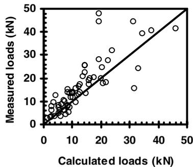
Figure 2. Comparing measured and calculated loads for steel strips.
