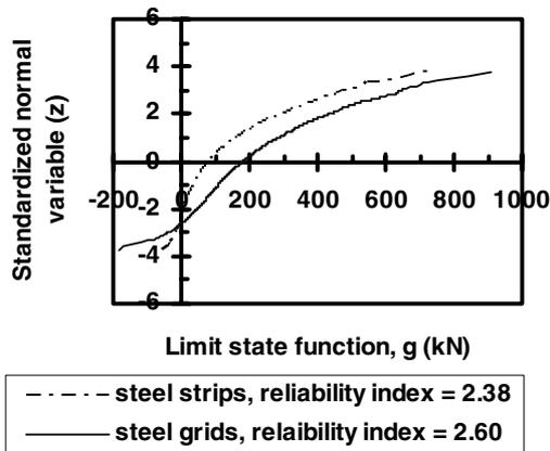
Figure 4. Monte Carlo analysis results for pullout resistance of steel reinforcements ( $\gamma = 1.35$  and  $\phi = 0.9$ ).
