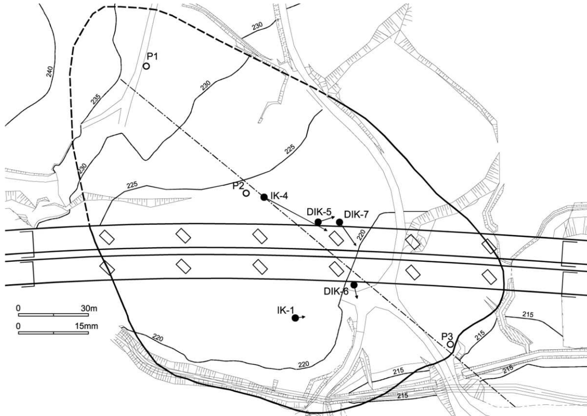
Figure 1. Viaducts, pier foundations, contours of the landslide, positions of inclinometers (IK), deformaters + inclinometers (DIK), piezometers (P) and total horizontal displacement vectors at ground surface measured by inclinometers up to February 2009
