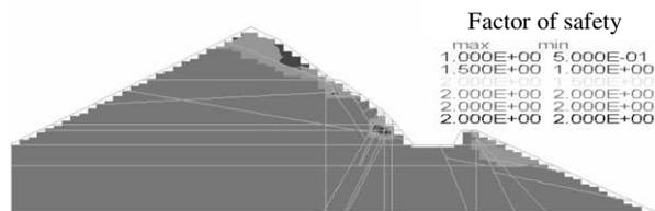
Figure 8. Factor of safety affected by damage index
