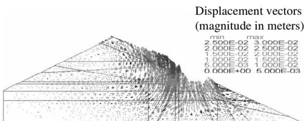
4.1 Figure 5. Displacement vectors at maximum slope section
