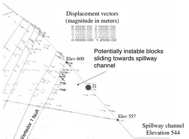
Figure 11. Detail of displacements at slope's toe for design earthquake
