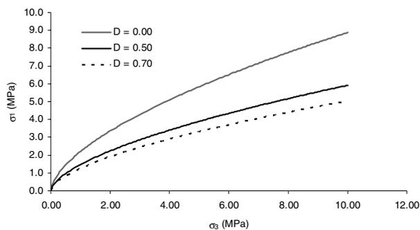
Figure 7. Hoek and Brown failure envelopes for rock mass damage
