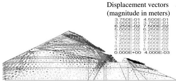
Figure 10. Relative displacements at the end of design earthquake
