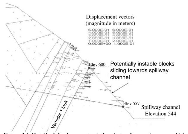
Figure 14. Detail of displacements at slope's toe for maximum credible earthquake (Tr10000)
