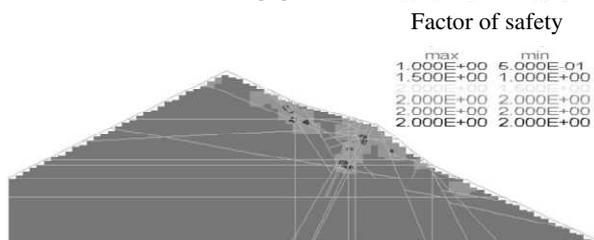
Figure 4. Security factor before excavation in maximum section
