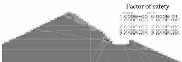
Figure 6. Security factor at maximum slope section
