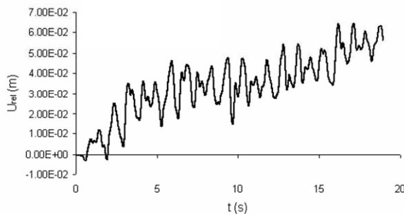
Figure 12. Displacement evolution at point B during design earthquake
