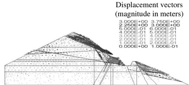
Figure 13. Relative displacements at the end of Tr10000 earthquake
