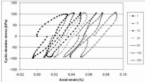
Figure1. Hysteresis loops for test on sample with M.A.S.=25.4 mm, b=5%,  $\sigma_3=200$  kPa,  $\sigma_d=200$  kPa, T=25°C
