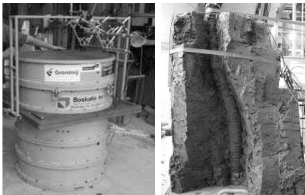
Figure 4. Large-scale Direct Shear test on nails in clay
