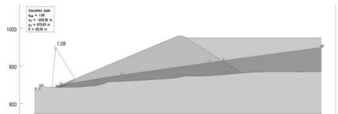
Figure 8. Designed condition without drainage
