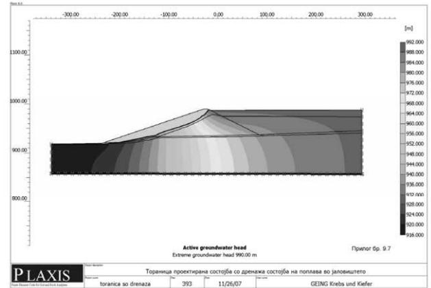
Figure 6. Designed condition with drainage for flooding of the tailing dam
