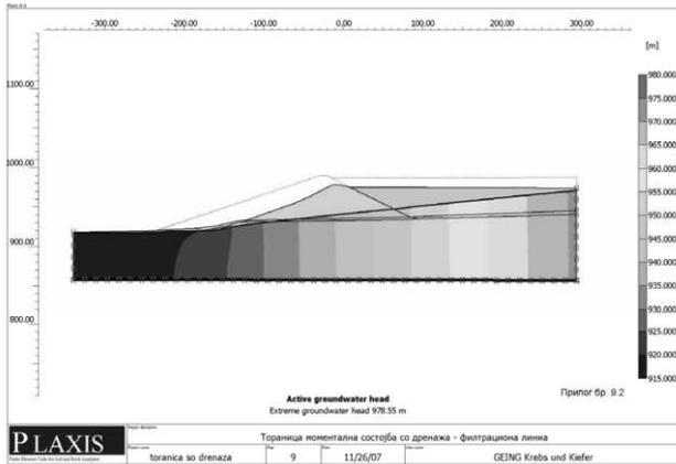
Figure 3. Filtration line during normal regime of work with drainage
