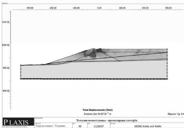
Figure 4. Total displacements - designed condition without drainage
