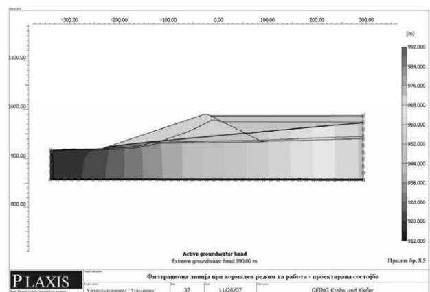
Figure 2. Filtration line during normal regime of work without drainage
