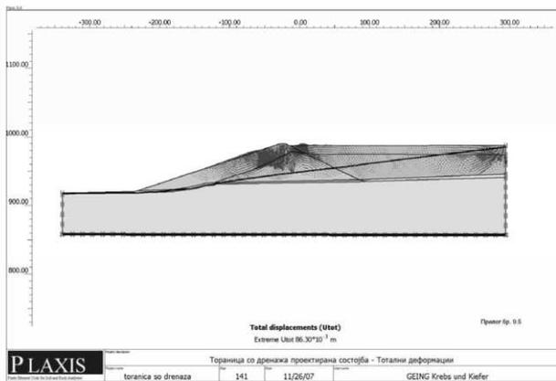
Figure 5. Total displacements - designed condition with drainage
