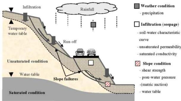
Figure 1. Mechanism of rainfall-induced slope failure
