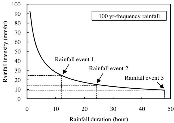
Figure 5. Rainfall intensity-duration curve for 100 yrs frequency
