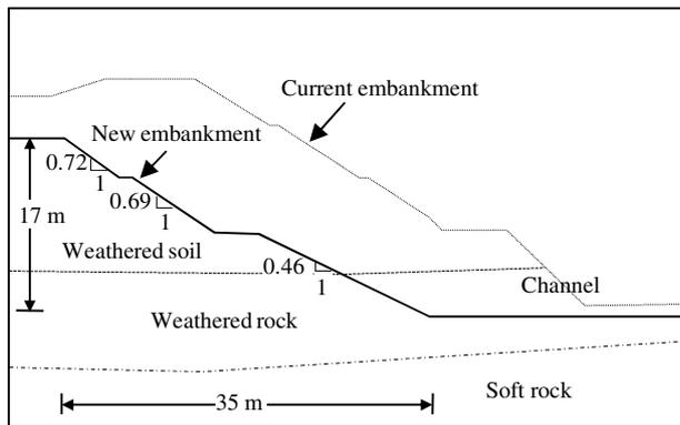
Figure 2. Geometry of new embankment
