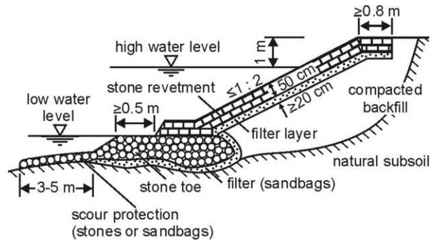
Figure 2. Characteristic cross section of the river bank protection.
