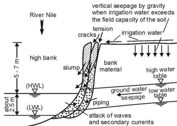
Figure 1. Factors affecting bank failure on the River Nile (NRI 1992).
