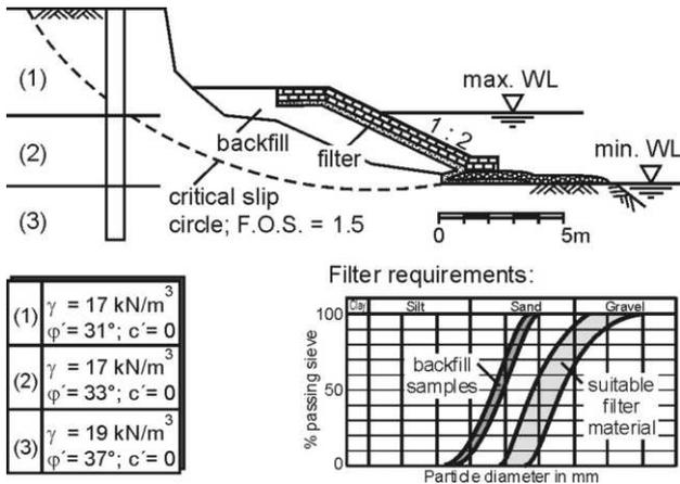
Figure 3. Exemplary cross section of the bank protection, designed in accordance with the guidelines.
