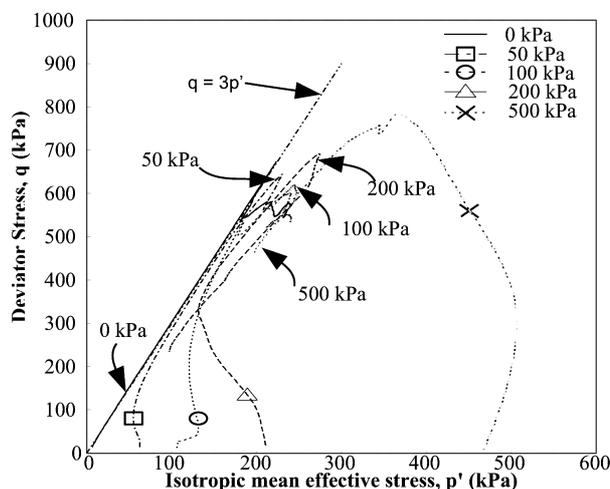
Figure 5. Stress path of triaxial test on 11 year old CB 'block' sample
