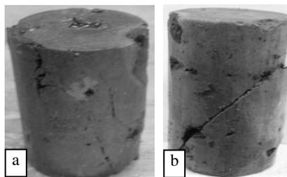
Figure 6 Triaxial specimens after test (a)  $\sigma_3'=50\text{kPa}$  (b)  $\sigma_3'=500\text{kPa}$
