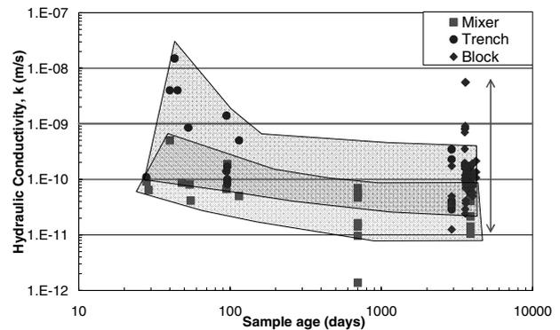
Figure 2. Hydraulic conductivity result with time for CB samples
