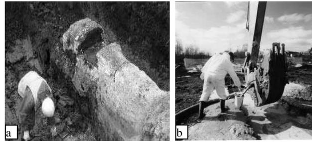
Figure 1. a) Excavation of 'block' field sample b) Slurry collection to prepare 'trench-cast' sample
