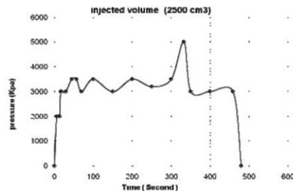
Fig (5) pressure time relationship at discharge rate = 0.32 l/min.
