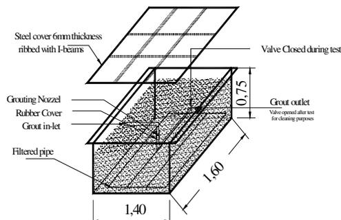
Fig (1) schematic drawing for the tank with internal dimensions.
