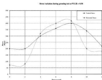
Fig (4) total stress variation during injection at W.S.R = 0.50
