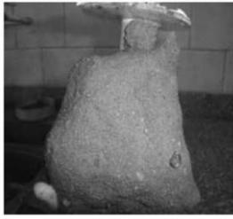
Fig (2) Grout bulb, Test No. (5), Discharge rate = 0.32 L/min and water solid ratio = 0.50
