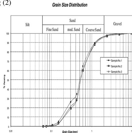
Figure (2) Grain size distribution for Tested Sand
