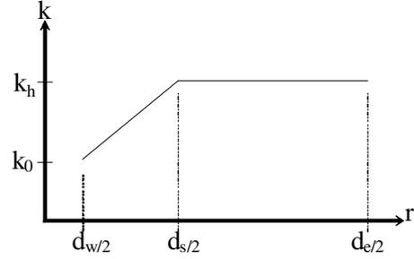
Figure 3. Linear variation of permeability in the smear zone
