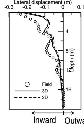
Figure 10. Lateral displacements at embankment toe at 168<sup>th</sup> day
