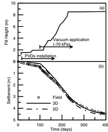
Figure 11. (a) Loading history and (b) Consolidation settlements for Settlement plate SP-12
