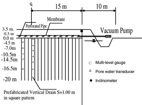
Figure 6. Cross-section of an embankment with field instrumentation
