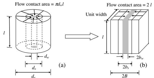
Figure 4. Unit cell analysis: (a) axisymmetric condition, (b) equivalent plane strain condition (after Indraratna et al., 2005)
