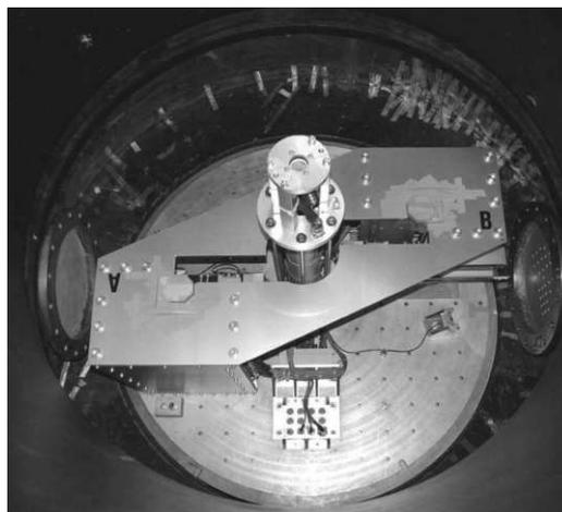
Figure 3. Drum centrifuge (2.2 m drum diameter) arrangement
