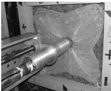
Figure 5. Falling weight resting on geotextile after 10 impacts at 20g
