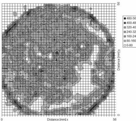
Figure 10. Stress distribution at displacement of 18 mm in the test 3.2\_dtv model B
