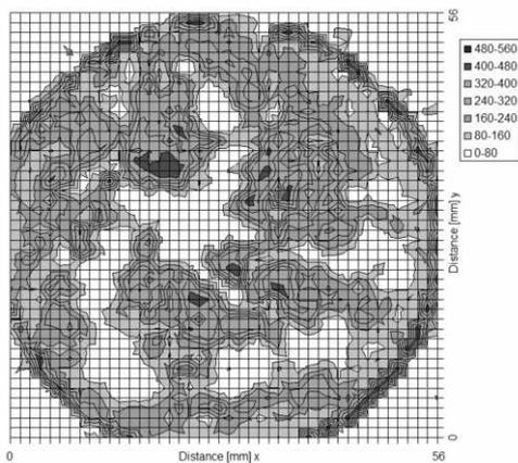
Figure 9. Stress distribution at displacement of 18 mm in the test 3.2\_dtv model A
