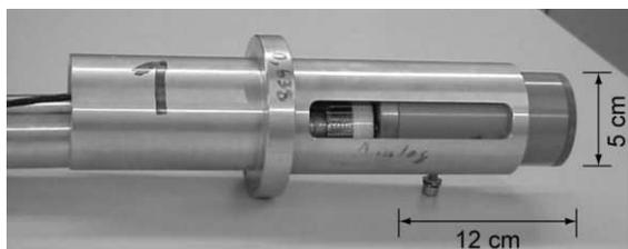
Figure 2. Dynamic compaction tool. (photograph Markus Iten)
