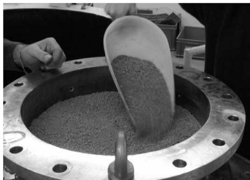
Figure 4. Placement of dry model lumps in the cylindrical container, 40 cm in diameter (photograph Jan Najser)
