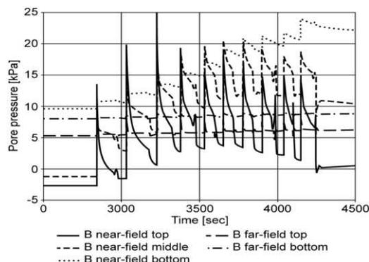
Figure 7. Pore pressure variations during 10 impact events for 3.2\_dtv model B, with nominal 2.7 kJ impact energy
