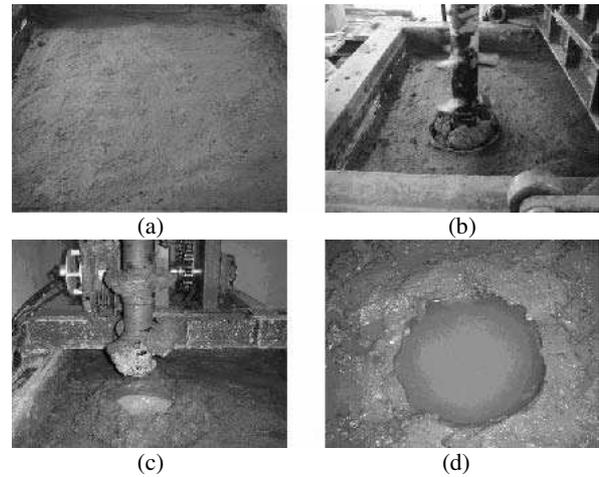
Fig. 2 Test Process; a) Filling soils in container, b) Rotational insertion by the shaft of experimental box, c) Mixing of admixture, d) Curing of improved column
