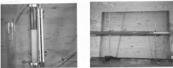
a. Clean sand packed in the model and ready for experiment. b. Sand saturated with red colored water.
