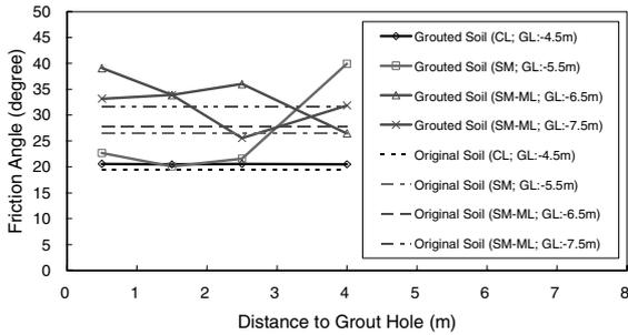
Figure 5. Friction angles of grouted soils.
