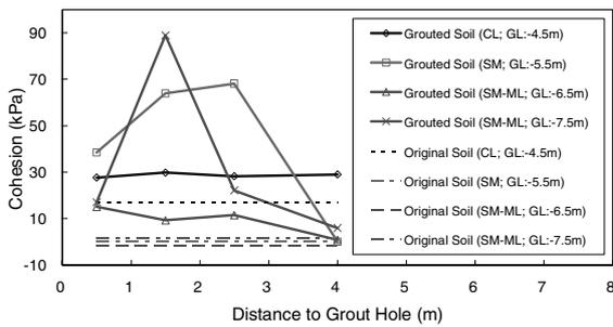
Figure 6. Cohesions of grouted soils.
