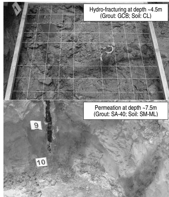
Figure 3. Observed mechanisms of grout injection.
