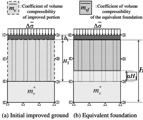
Figure 5. Concept of equivalent conversion ratio  $\alpha$ .
