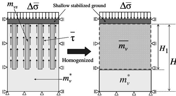
Figure 3. Concept of the homogenized composite ground.
