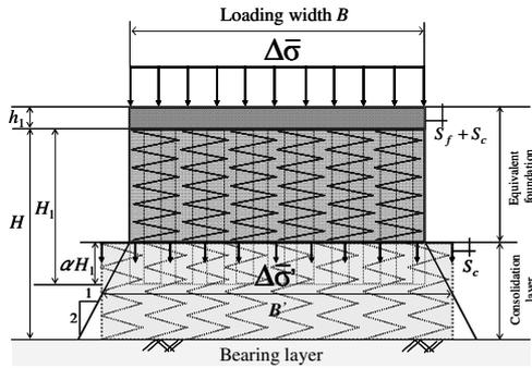
Figure 8. Concept for estimation of the total settlement.
