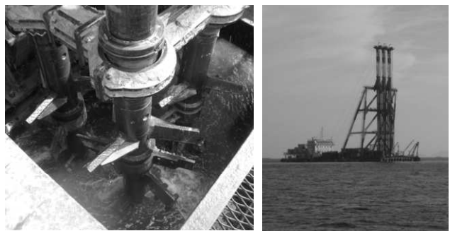
Figure 4. Mixing blades of the deep mixing machine and offshore CDM production barge.
