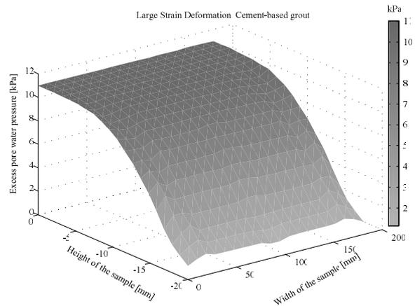
Figure 2. Excess pore water pressure (large deformation).
