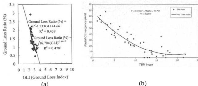
Figure 3. (a) Ground Loss Ratio versus Ground Loss Index according to Chang et al. (2000). (b) The relationship between  $I_{\text{TBM}}$  and Tunnel Radial Convergence for different areas of the Ghomroud tunnel excavated length, according to Farrock & Rostami (2008).
