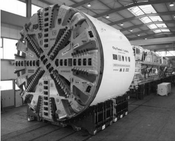
Figure 1 Tunnel Boring Machine.
