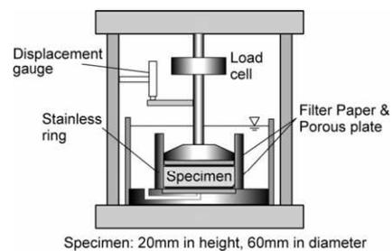
Figure 2 Testing apparatus for measuring the swelling pressure
