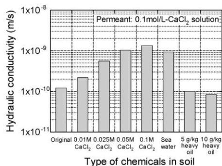
Figure 4 Effect of the chemicals in the soil pore water on the  $k$ .
