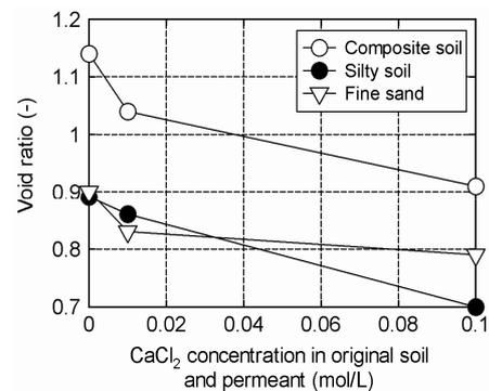
Figure 6 Effects of the  $\text{CaCl}_2$  concentration on the void ratio of the SB
