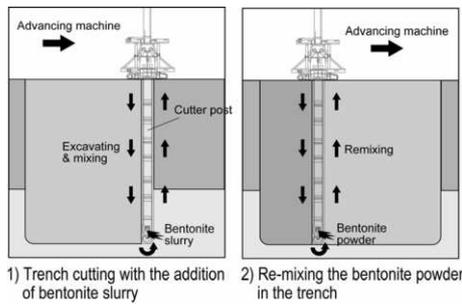
Figure 1 In situ construction of SB vertical cut-off wall by TRD method
