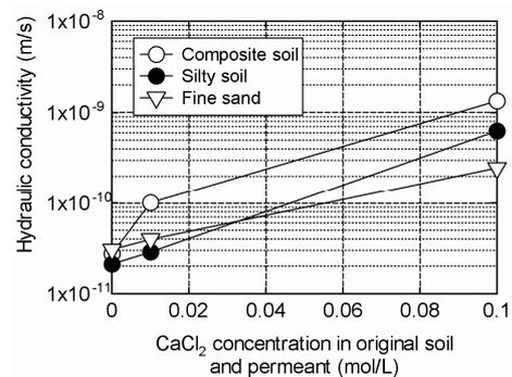
Figure 5 Effects of the  $\text{CaCl}_2$  concentration on the  $k$
