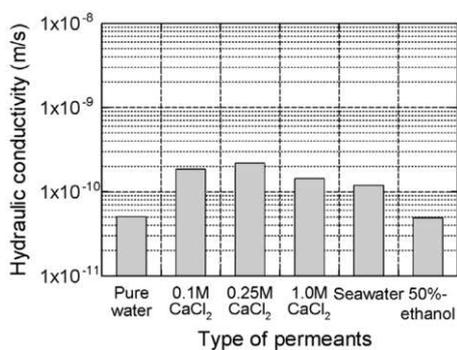
Figure 3 Effect of the chemicals in the permeant on the  $k$ .
