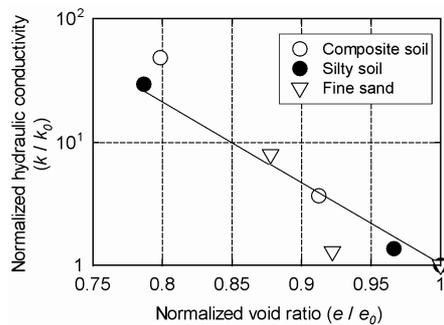
Figure 7 Normalized void ratio vs.  $k$  values
