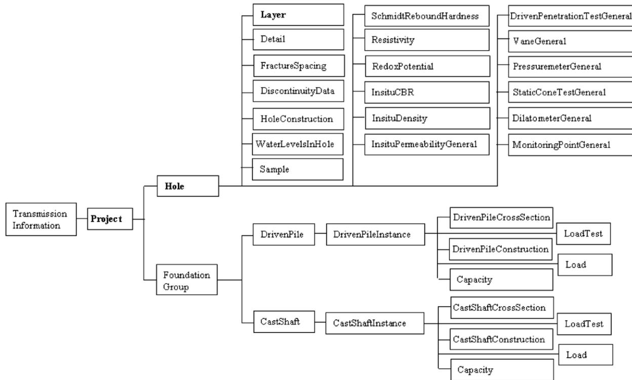
Figure 1. Data structure for DIGGS based on DIGGS, 2006 and Styler et al, 2007 (Toll, 2007a)
