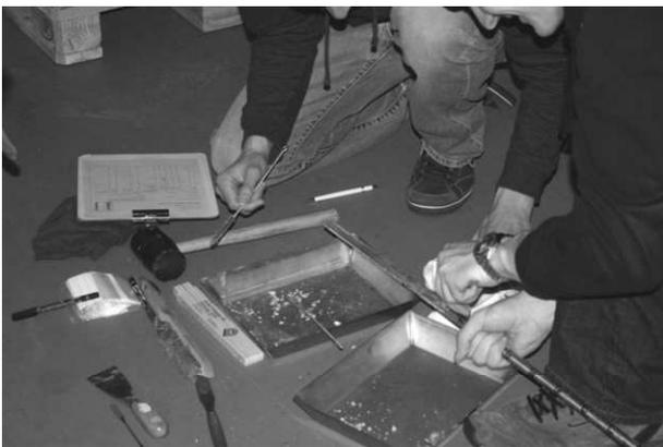
Figure 7. Students emptying the slotted rod and storing the samples in bags for further evaluation.
