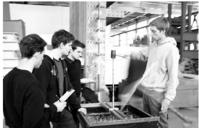
Figure 4. Students driving the sampler into the model.
